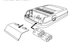
Press down on the battery compartment cover and slide it off in the direction of the arrow on the cover. 2. Install the batteries as indicated by the polarity symbols (+ and –) marked inside the compartment.
